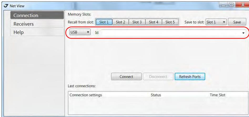
**Figure 1-6. NetView - Connection via USB port**
