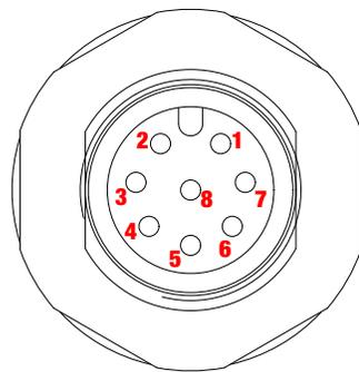
**Figure A-6. RS422/RS232/CAN Connector**
