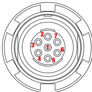
**Figure A-5. Ethernet Connector**
