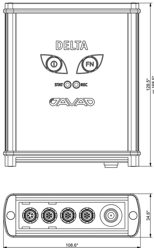
**Figure 1-2. DELTA dimensions in mm**
