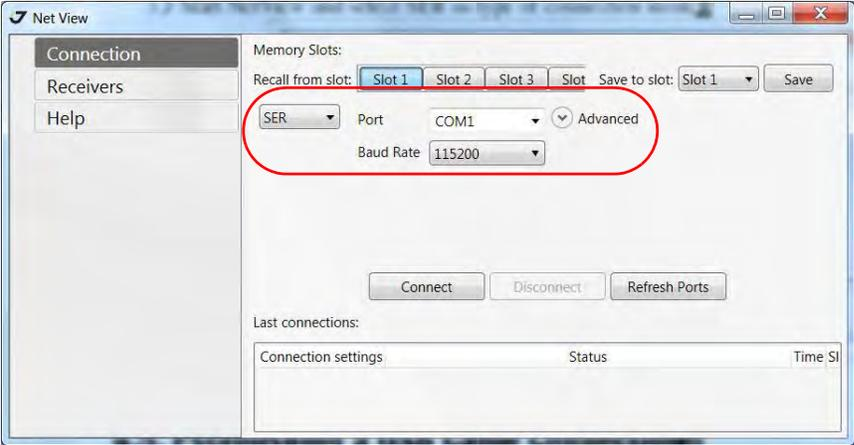
**Figure 1-5. NetView - Connection via serial port**
