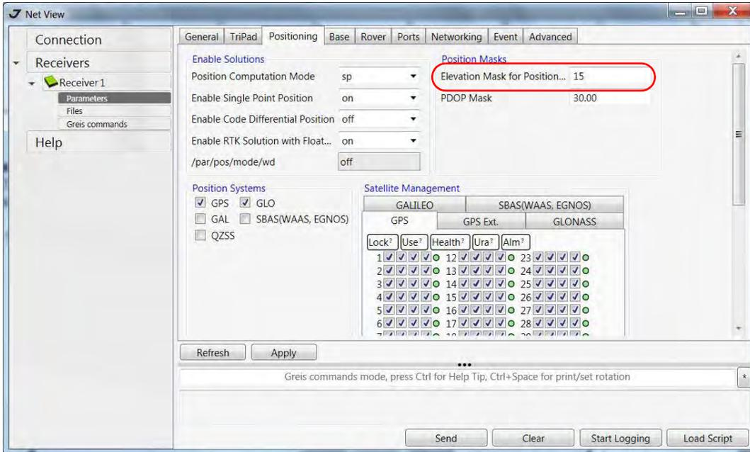
**Figure 1-9. Positioning tab - Elevation Mask**
