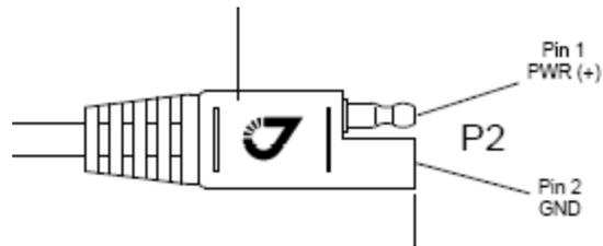
**Figure A-2. Polarity of SAE for power cable P/N 14-578101-01**
